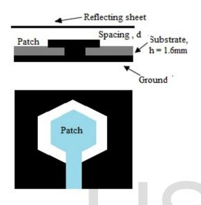
Figure1. Geometry of Proposed Antenna
