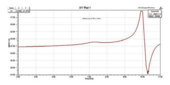
Figure 3. Return Loss - Proposed antenna
