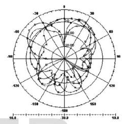
Figure 6. Radiation pattern of the antenna with reflecting sheet on the back.
